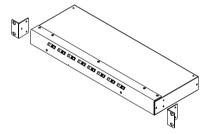
3. Slide the unit into the rack and secure it to the rack.
