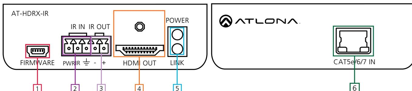
1. Firmware Update Port: Use a Mini USB to USB cable to connect to a Windows computer for updating.
