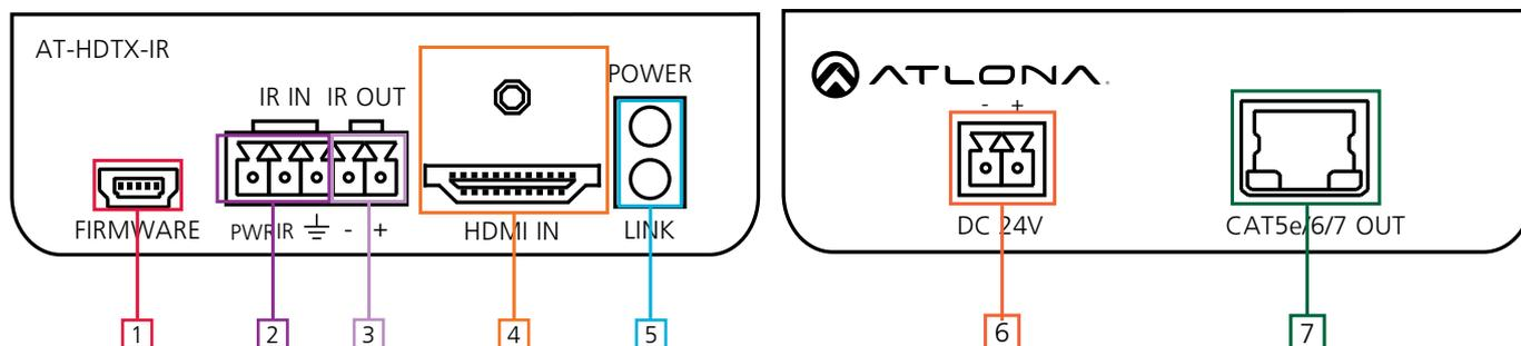
1. Firmware Update Port: Use a Mini USB to USB A cable to connect to a Windows computer for updating.
