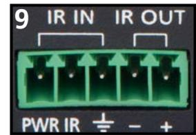
To ensure the power cable isn't too long, a captive screw connector has been included. The pin out (see picture 10) and the wire configuration (see picture 11 and 12) are shown below. \*Power used with transmitters only\*
