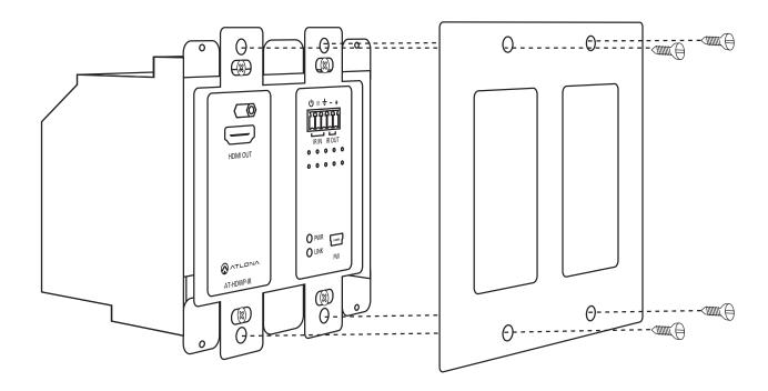
Install the Decora face plate over the Decora HDBaseT module using the four remaining screws (these screws will have painted white heads).
