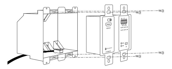
The first step in installation is to connect the cat cable to the Decora HDBaseT module and install it into the electrical box (as seen above).
