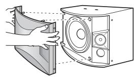
To reattach, do these steps in reverse order. The 4 pegs inside the grille should be set in the corresponding holes on the speaker.
