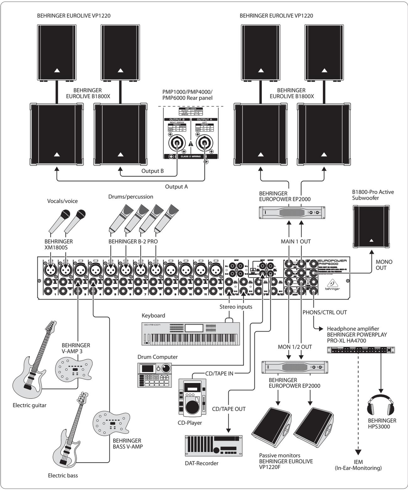
Fig. 5.5: Expanded set-up
