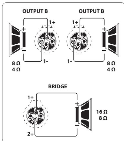
Fig. 4.7: Pin assignment
