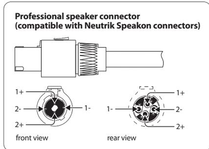
Fig. 4.6: Professional speaker connector with polarity allocation
