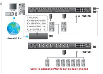
\* The CN6000 from ATEN is an ultra-compact, Over IP solution for remote access to computers and KVM installations. Please refer to www.aten.com for more details.
