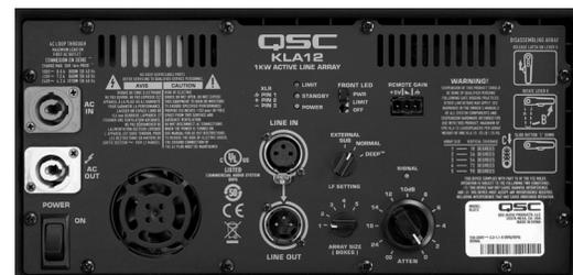
In an installed application, multiple KLA Series loudspeakers can be "daisy-chained" for total gain control from a single remote pot wired to the on-board Phoenix-style connector. Additional power module characteristics on KLA include a balanced, line-level XLR input in parallel with an XLR "Thru" connector, powerCON® In and Thru connectors, Attenuation Control and LED indicators for Signal and Limit, as well as discrete LED indicators for Power/Standby status.
