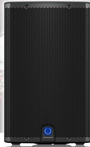
The 2,500-Watt iQ12 is a powered two-way loudspeaker ideally suited for a wide range of portable and fixed installation, music and speech sound reinforcement applications. The driver complement includes an 12" low frequency driver with a low mass voice coil for improved transient response, and a high temperature 1" compression driver with copper-clad aluminium voice coil for extended high frequency reproduction.
