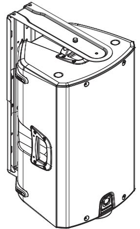
iQ12-WB wall bracket: vertical mounting.
